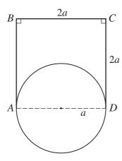
Three identical uniform rods, AB, BC and CD, each of mass M and length 2a, are rigidly joined to form three sides of a square. A uniform circular disc, of mass  $\frac{2}{3}M$  and radius a, has the opposite ends of one of its diameters attached to A and D respectively. The disc and the rods all lie in the same plane (see diagram). Find the moment of inertia of the system about the axis AD.
